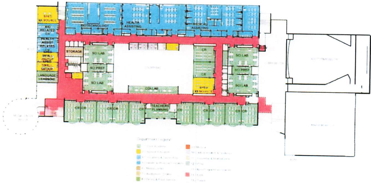
Typical floor layout for floors 2-4. Highlight of the layout includes CVTE spaces on the north side, traditional classrooms on the south side, science classrooms in the middle, and specialized spaces on the wings.
