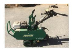
This is a Ryan 18" Jr. Sod Cutter, which is used for turf renovation and sod cutting. We can use this for trimming the sod around in-fields, and in growing and transferring our own sod for patching. It can be used for trenching, cabling or piping. This equipment was made possible by a grant from the Piccolo Family Charitable Foundation.
