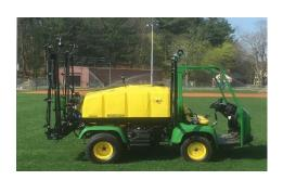
One such attachment is the John Deere HD300 SelectSpray shown here. It is used in the application of fertilizer, insect control and herbicides. This equipment was made possible by a grant from the Piccolo Family Charitable Foundation.
