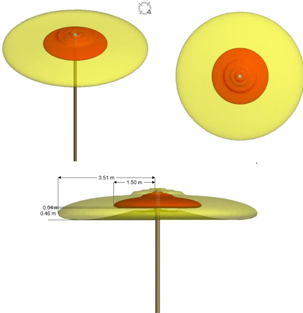
Figure 6 VVSSP-360S-F Compliance Boundary / Pattern Oblique, Overhead, & Side Views
