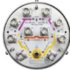
10-port small cell antenna, 4x 1695–2690, 4x 3400–3800 and 2x 5150–5925 MHz. 65° HPBW, Internal RET and SBT
