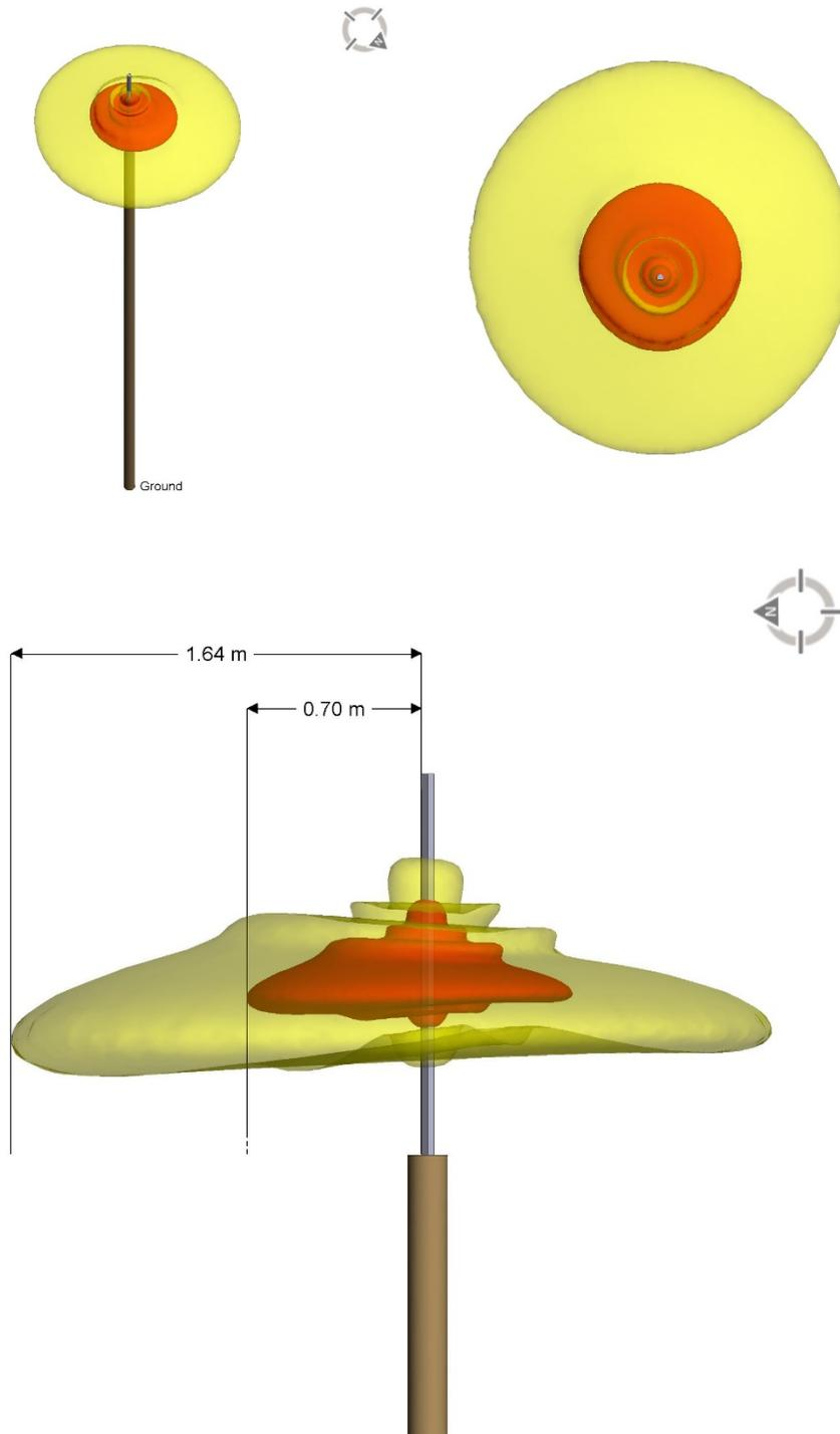
Figure 7 GO6010-07078 Compliance Boundary / Pattern Oblique, Overhead, & Side Views
