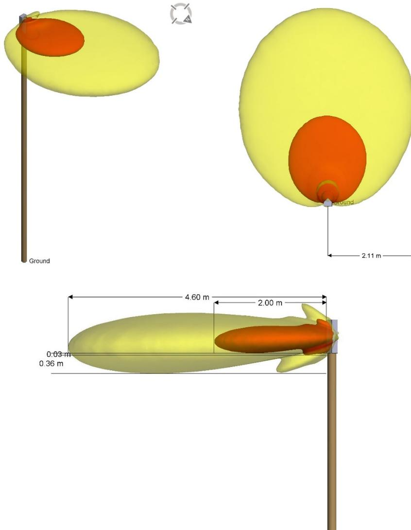
Figure 4 VVSSP-65S-R1B-4455 Compliance Boundary / Pattern Oblique, Overhead, & Side Views
