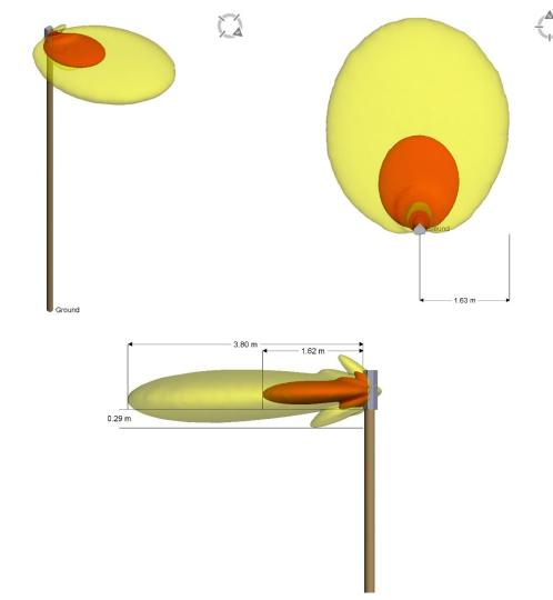
Figure 5 VVSSP-65S-R1B-4402 Compliance Boundary / Pattern Oblique, Overhead, & Side Views
