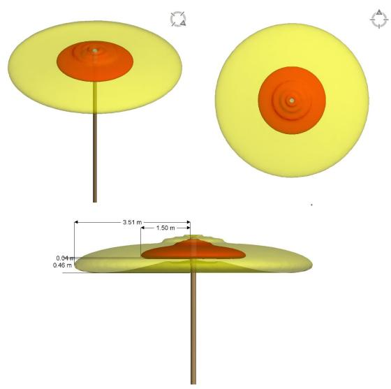
Figure 6 VVSSP-360S-F Compliance Boundary / Pattern Oblique, Overhead, & Side Views
