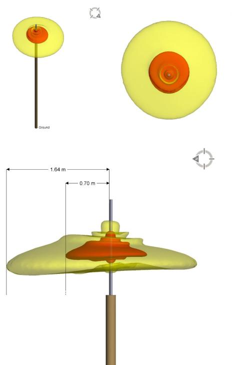
Figure 7 GO6010-07078 Compliance Boundary / Pattern Oblique, Overhead, & Side Views
