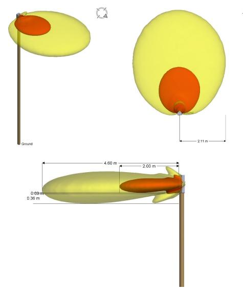
Figure 4 VVSSP-65S-R1B-4455 Compliance Boundary / Pattern Oblique, Overhead, & Side Views
